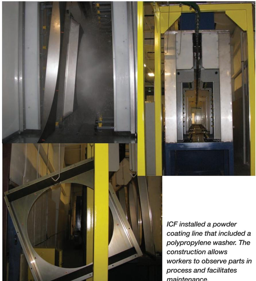
*ICF installed a powder coating line that included a polypropylene washer. The construction allows workers to observe parts in process and facilitates maintenance.*
